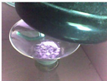
Figure 1. Irradiation with a mercury UV lamp of 60 W maintaining an air flow of 6 l/min through the photocatalyst for 48 hours.
